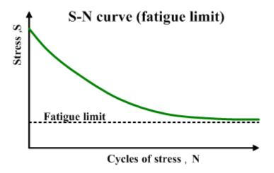
The tests results are presented in form of S-N curve (stress vs. number of cycles):
