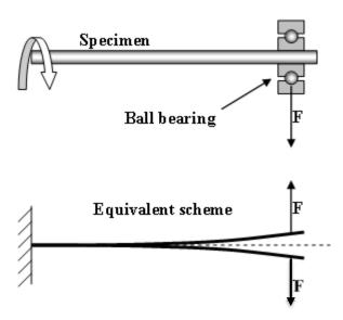
Fatigue strength at N cycles is the load, producing the material fracture after N cycling applications of the load.
